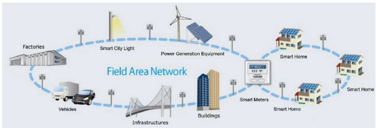
Figure 8: Example of FAN (Field Area Network) [FAN] Courtesy of Kyoto University, Nissin Systems, ROHM
